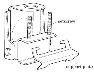
①Loosen the setscrews and remove the setscrews and insert the support plate in the bracket.
