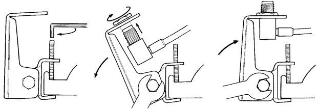
(1) Fix the bracket on a roofside gutter with the attached hexagonal wrench.
