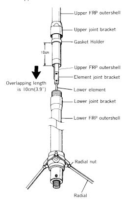
2) Put lower element into element joint bracket thoroughly and fix it.
